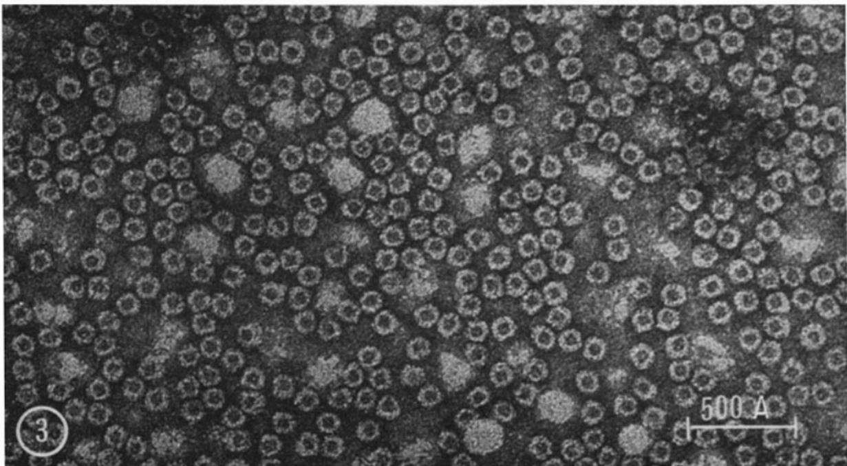
Apoferritin negatively stained with uranyl acetate. Image collected on a Phillips EM 200 operating at 80 kV. This is the sample I am using to plunge and prepare cryo grids for screening.
