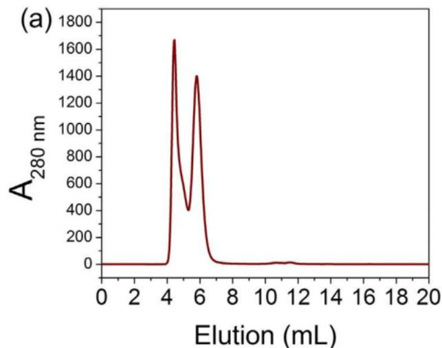
Size exclusion chromatogram of commercial equine spleen ferritin at pH 4.5 using a SupelCo column on an Akta Purifier 900. Absorbance measured at 280 nm.
